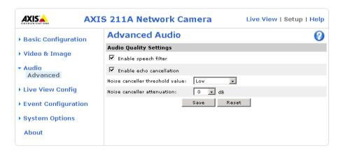
Enable speech filter improves the sound quality when the microphone is placed close to the person talking and can also help reduce background noise. The filter cuts the lowest and the highest frequencies. The bypass frequency range is approximately 250Hz to 3700Hz (measured at -10dB cut-off break points).
